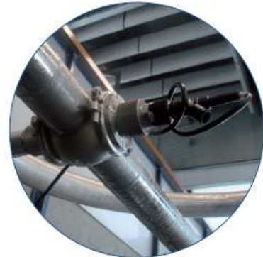
Fig. 1: M1100 sensor in use between tank and filler in a 60 mm line.
