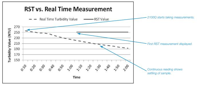
Although the sample continuously settles out of solution, the RST calculated value does not change. No more guessing and no more replicate runs—you get the right answer every time.
