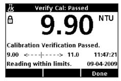
Be confident in your measurement by running the quick and easy Verify Cal function using the included 10 NTU StablCal primary standard.
