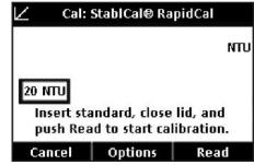
In the range up to 40 NTU, the single standard RapidCal calibration mode reduces calibration complexity by eliminating multiple standard full calibrations. You save time and ensure you meet reporting requirements.
